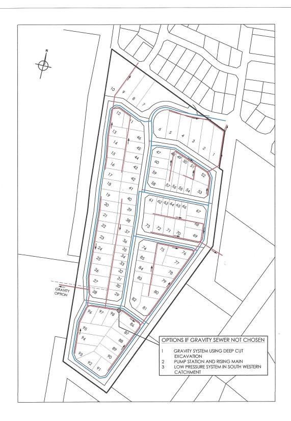
GRAVITY SEWER THROUGH THE MILNE FARM. SEE PLAN No 2 FOR DETAILS  $\label{eq:control} % \begin{array}{ll} \text{ The properties of the p$
